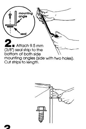
Attach side-mounting angle with two, hex-head, metal screws using 6.4 mm (1/4") socket and socket wrench or 1/4" nut driver.
